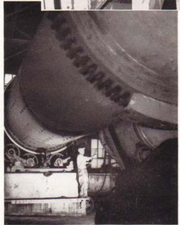
The final treatment of the fine coal is in these large heated cylinders in the heat drying plant. The coal gets a hot ride in these 65 foot long cylinders—about 800° F in the shade. Domenico Milchiorre, Heat Dryer Operator, has been at Champion I since 1930.
