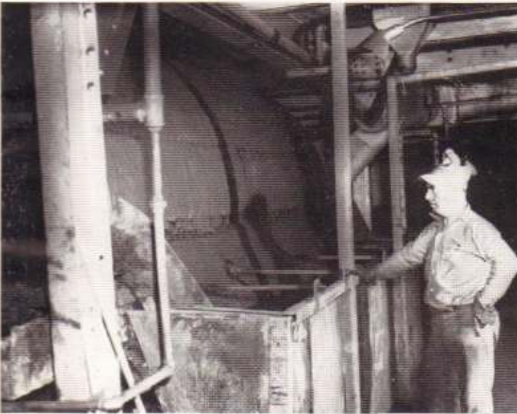
Charles Smith, Filter Operator, is watching the fine coal come off the Oliver filter. A rotating 14 foot drum covered with cloth picks up the fine coal and the moisture is sucked out of the solution by a strong vacuum. There are three Oliver filters and each one can handle up to 14 tons per hour. The fine coal now goes to the heat drying plant.
