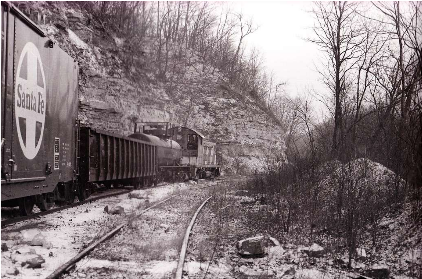
Engine 76 shoves freight cars on the Hill Track in 1980. Note rocks lying between the tracks and dirt filling the area between the rails. Photo by Roy Parkinson courtesy Gene P. Schaeffer.
