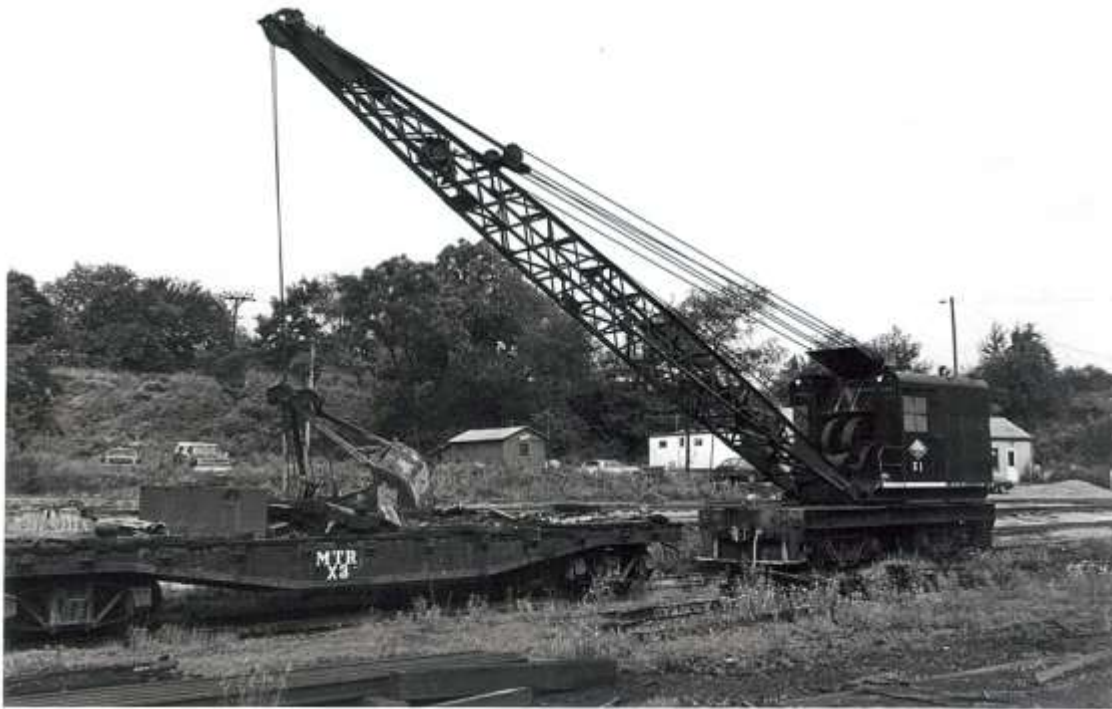
X1, accompanied by flat car X3, sits at Champion in 1981 while on a ditch clearing project. The clamshell bucket was being used for this job Gene P. Schaeffer photo
