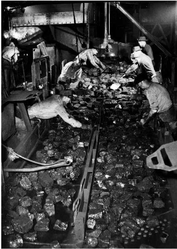
A picking table, where workers hand-picked impurities out of Green Coal. John Collier photo in 1942.
