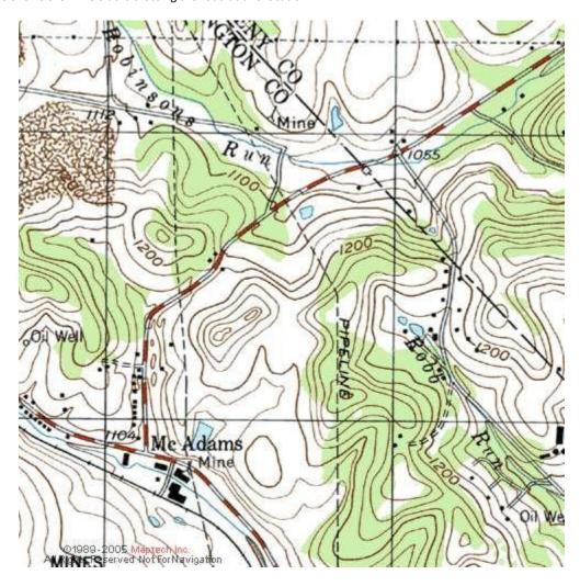
This close-up shows the trestle where the mine trains for Montour No. 9 crossed Donaldson Road to enter the second hill. The entry to the southwest became a major source of acid mine drainage as shown in the next photo for the Operation Scarlift Report for Robinson Run.
