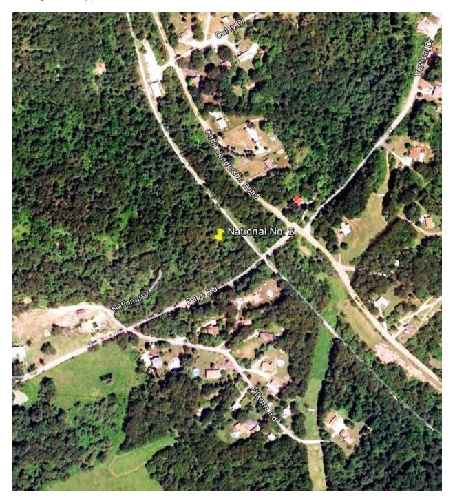
This topographic map shows the location of the two shafts at National No. 2. The shaft next to the word "Mine" was the production shaft and the shaft above the mine dump would have been for ventilation, supplies, and probably an escape shaft.
