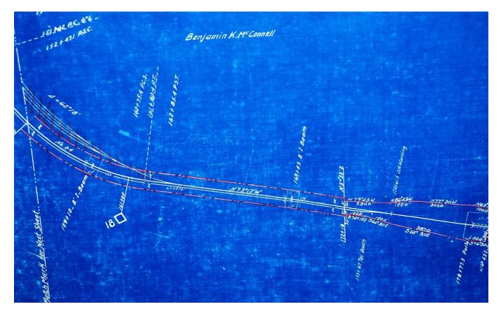
This blueprint shows the east end of the National No. 2 yard and the east end connection of National Siding to the main track. The tipple had the standard four-track loading features of most mines in this area for Lump, Egg, Nut, and Slack. The tipple centerline was located along the line drawn below the word "Mine" on the print.
