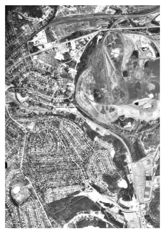
This 1930s era mine map shows two openings for Montour No. 8 Mine. Houses were built directly over the remaining mine entries that were left intact after the coal pillars were removed.
